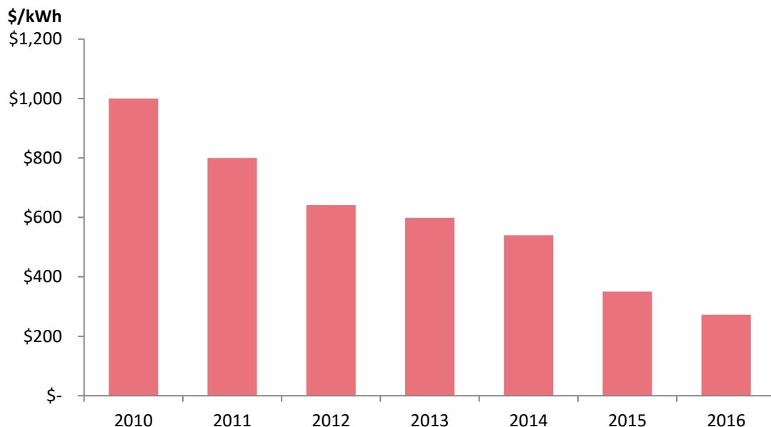
Figure 4: Lithium Ion Battery Costs<sup>6</sup>
